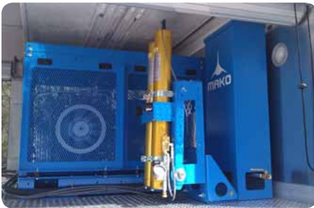
Fire Truck Filtration Delivers quality air to CGA Grade E standards
